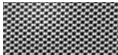
A scanning transmission electron microscopy image of a diamond. At this resolution you 'see' the individual dumbbells formed by two carbon atoms at the face centred cubic lattice points of the diamond structure. Jaco Olivier
