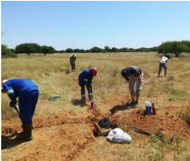
A moisture probe network consisting of eight sensors attached to a central unit has been installed at each site so that satellite-derived soil moisture data can be validated.
