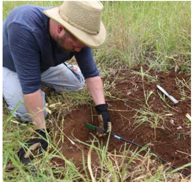
A moisture probe network consisting of eight sensors attached to a central unit has been installed at each site so that satellite-derived soil moisture data can be validated.
