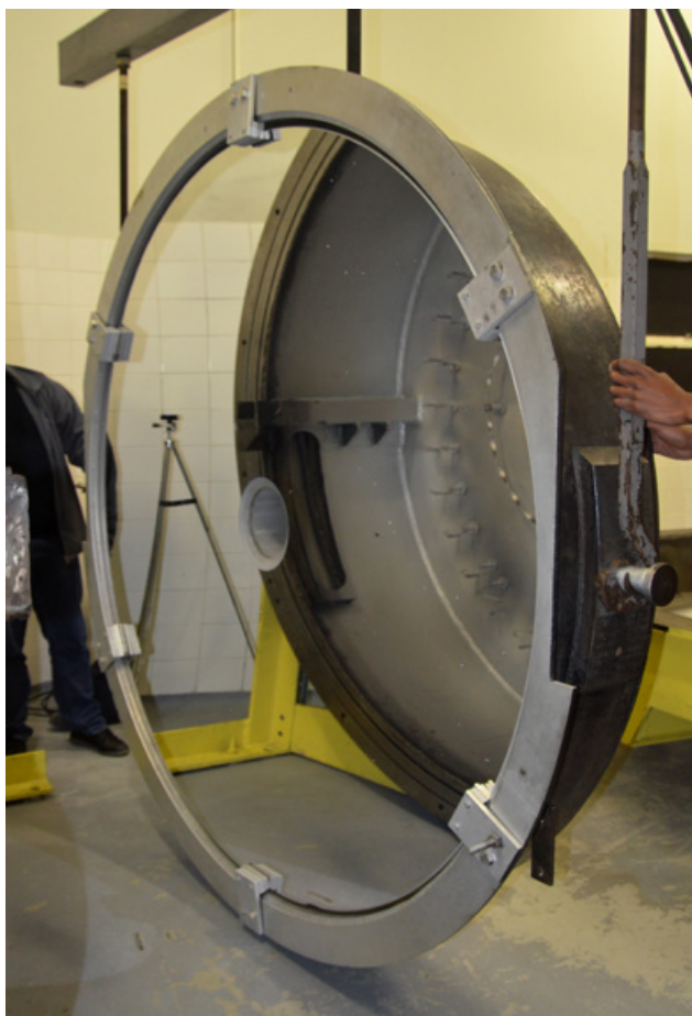
The freshly coated 74-inch primary mirror emerging from the aluminising tank. Lisa Crause
