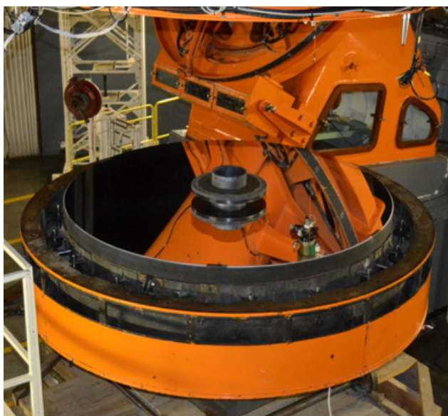
Installing the re-aluminised 74-inch primary mirror on the telescope. Lisa Crause
