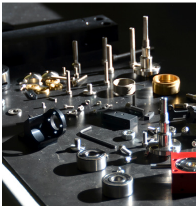
The SpUpNIC grating mechanism components prior to assembly. Lisa Crause
