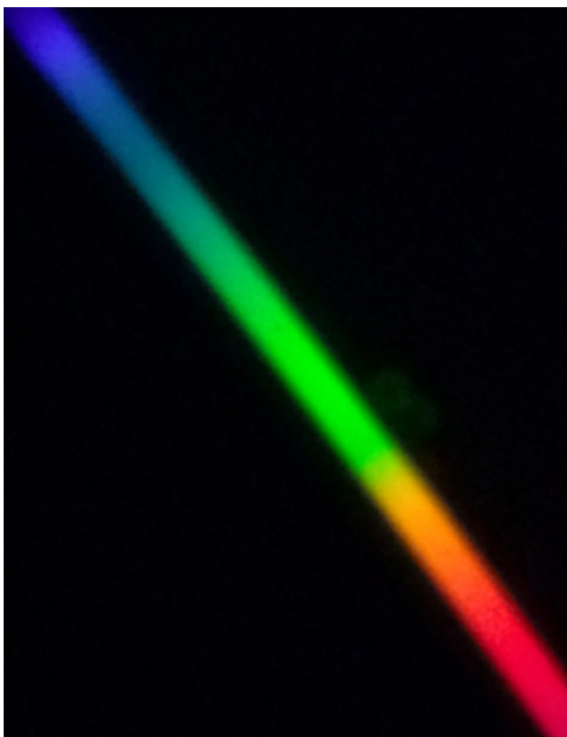
With the spectrograph optics aligned and white light injected through the slit, the new instrument produced its first spectrum.
