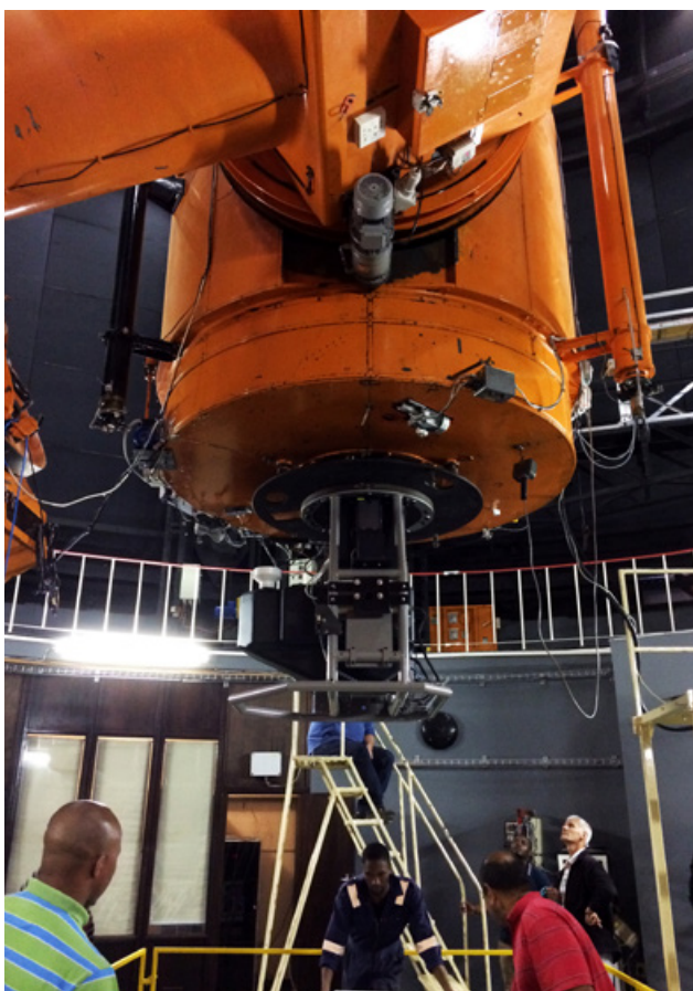
The upgraded Cassegrain spectrograph (SpUpNIC) being installed on the 74-inch on 21 October 2015 - first light was achieved that evening. Lisa Crause
