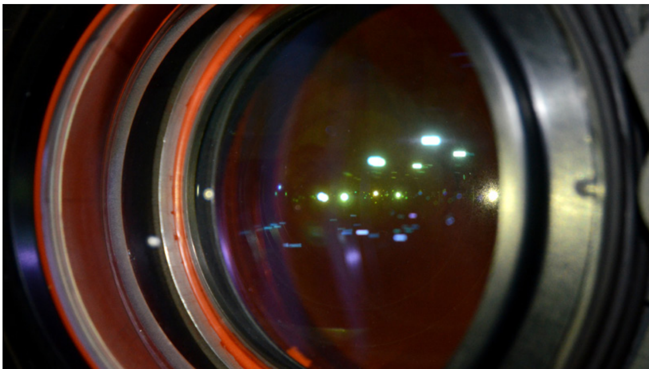
The SALTICAM lens barrel showing reflections from each of the optical surfaces in the system. Lisa Crause
