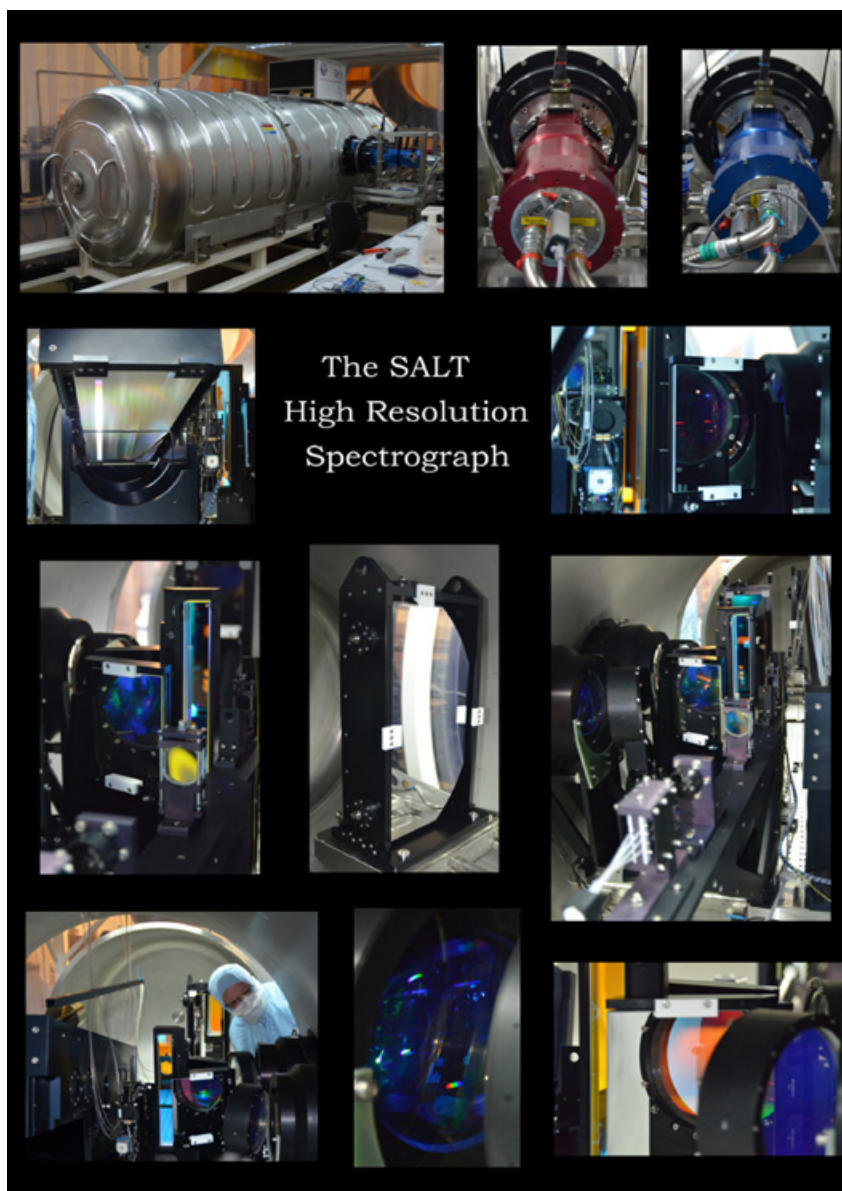
This collage shows various aspects of the high resolution spectrograph (HRS), including the 3-m long vacuum tank that encloses the optical bench, the red and blue camera units, the echelle grating and the numerous large mirrors and lenses. One needs to put on clean-room gear before working inside the tank as any contamination would compromise the integrity of the vacuum that shields the optics from thermal disruption. Lisa Crause
