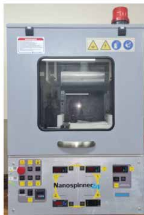
Figure 3: A conceptual diagram of nanofibres as brain implantable drug-loaded tissue-mimetic scaffolds (left) and the NanoSpinner24 machine used at the WADDP research unit for electrospinning of nanofibres (right)
