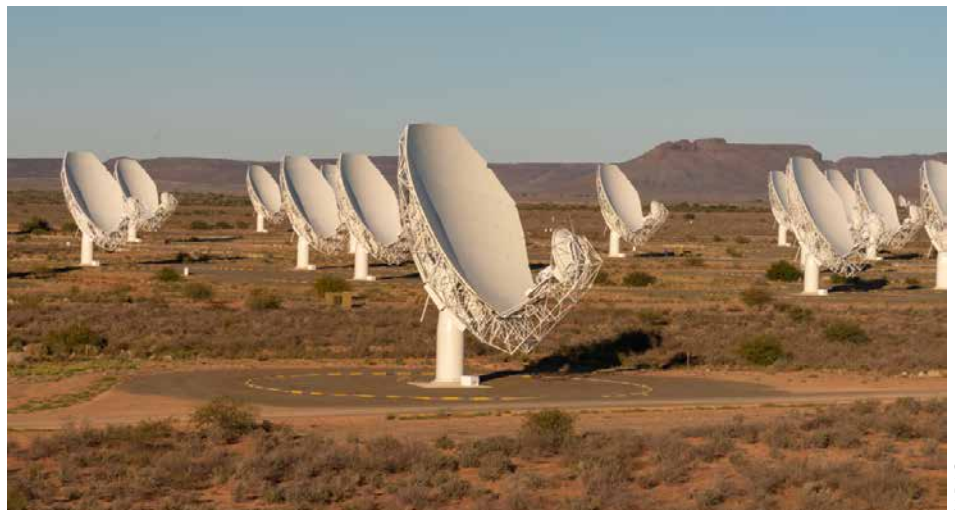
The MeerKAT telescope is an array of 64 interlinked receptors, each consisting of an antenna positioner (a steerable dish on a pedestal), a set of radio receivers, and associated digitisers and other electronics.
