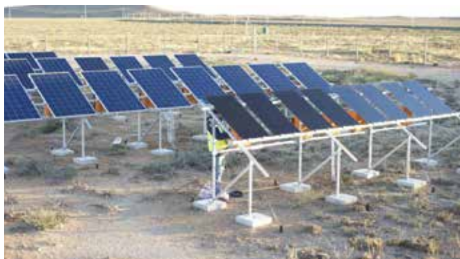
The PV system constructed for the research, with both stationary modules (left) and single-axis-trackers (right).
