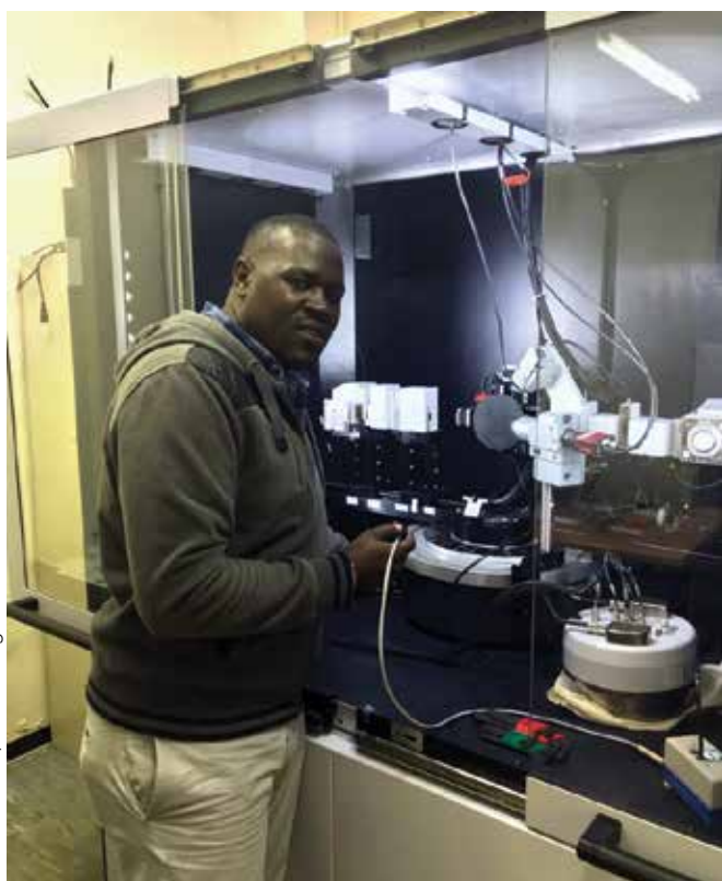
Francis in the laboratory at the Wits School of Chemistry, undertaking D10 Grazing Incidence X-ray diffraction. This technique is used to determine the phases of thin films at the sample surface and multi-layer films.
