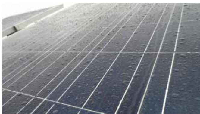
Application of a hydrophobic coating to the surface of PV modules caused large water droplets to accumulate (left), while water spread out uniformly on untreated PV modules (right).
