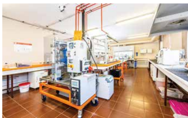
The HySA NWU team conducted extensive tests using this laboratory-scale hydrogenation system to assess the performance of dibenzyltoluene as a Liquid Organic Hydrogen Carrier (LOHC).
