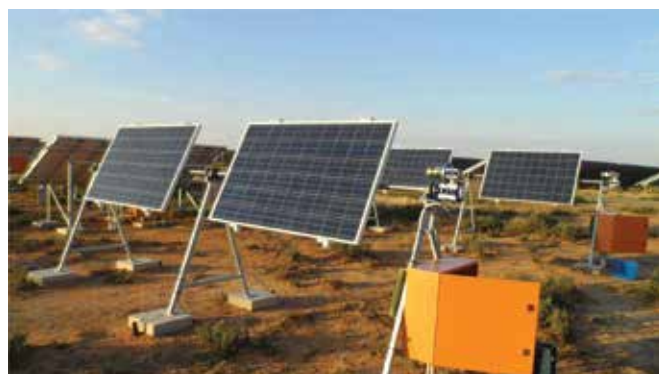
The PV system constructed for the research, with both stationary modules (left) and single-axis-trackers (right).
