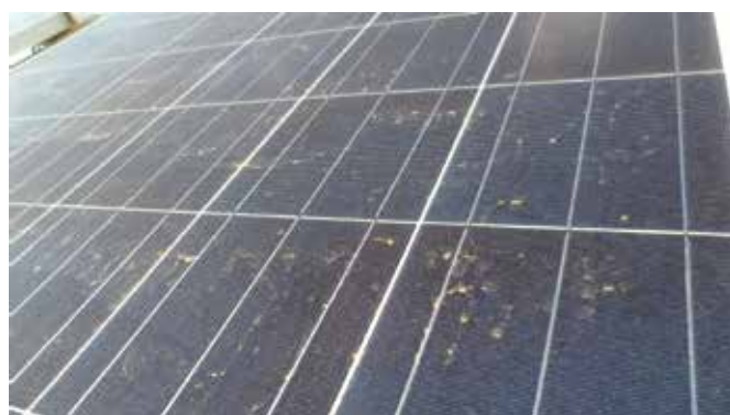
The hydrophobic coating caused small dust patches to form over time.
