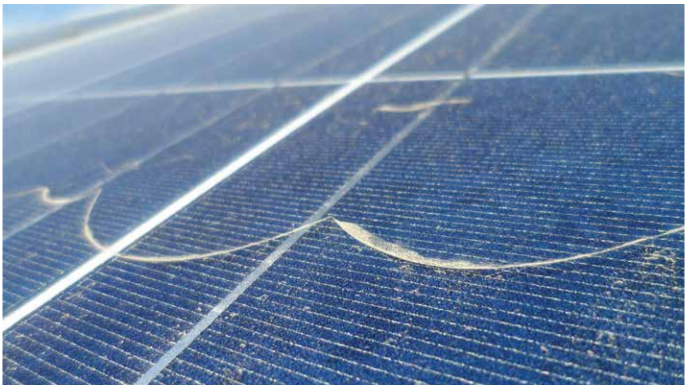
Rainfall at the study site was sometimes so light that it only shifted dust on the PV module surface, creating small wave-like dust lines.
