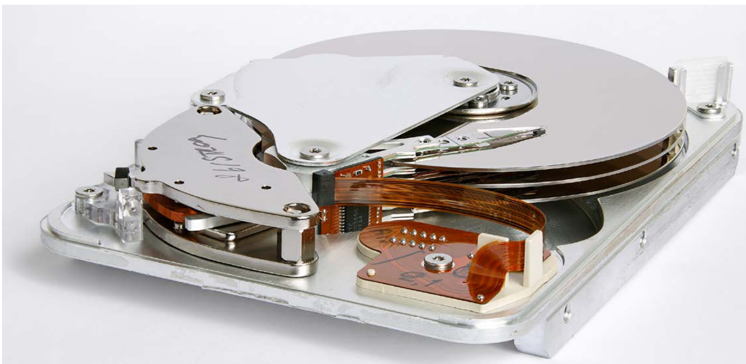
A Seagate 3.5-inch hard disk drive (HDD), showing the circular platters and read/write head mounted at the tip of the arm.
