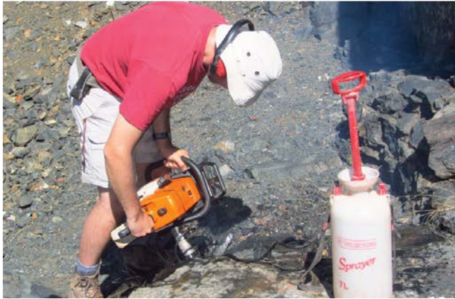
Palaeomagnetic core samples are collected from dolerite dykes, which are approximately 1 850 million years old.
