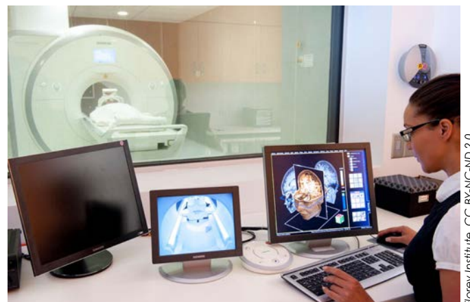
Advanced software allows greyscale MRI data to be visualised as colour 3D imagery.
