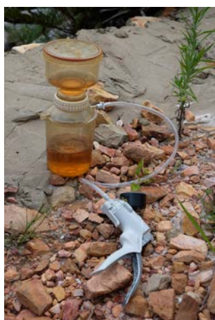
A handheld vacuum pump was used to filter water samples for laboratory analyses.
