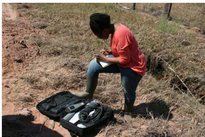
The pH, temperature, dissolved oxygen and conductivity of streams was measured with a multiprobe instrument.
