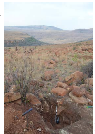
A lightproof tube is used to collect a sediment sample for luminescence dating once back in the laboratory.
