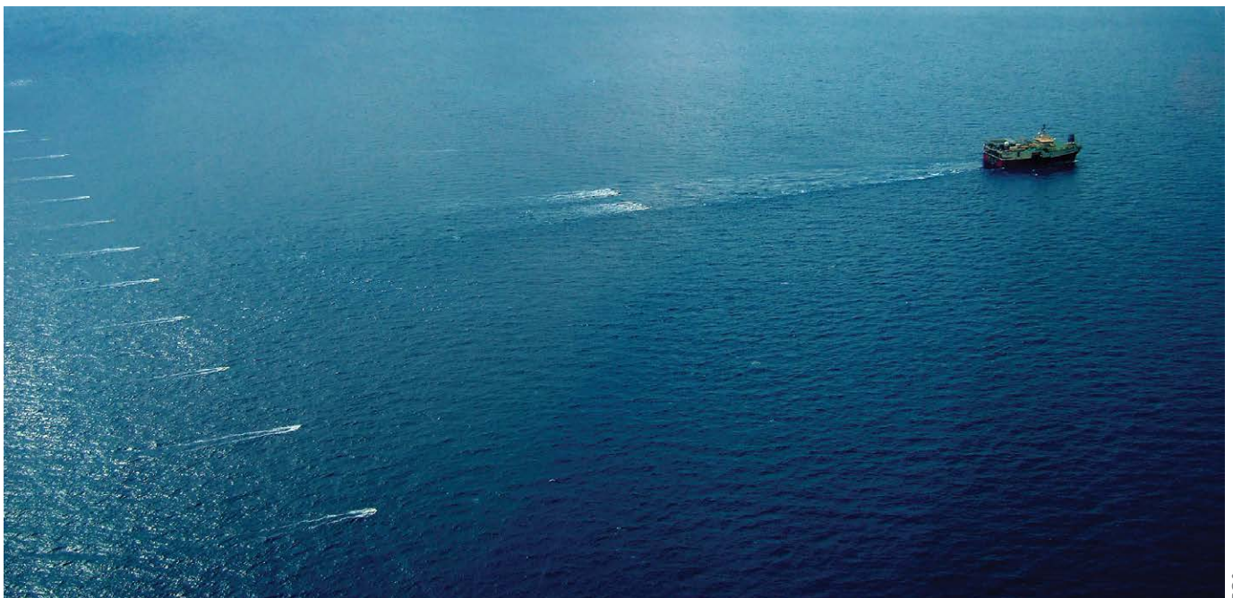
Seismic survey vessels tow airguns as well as the hydrophone-containing ‘streamers’ that may be up to 10 km long.
