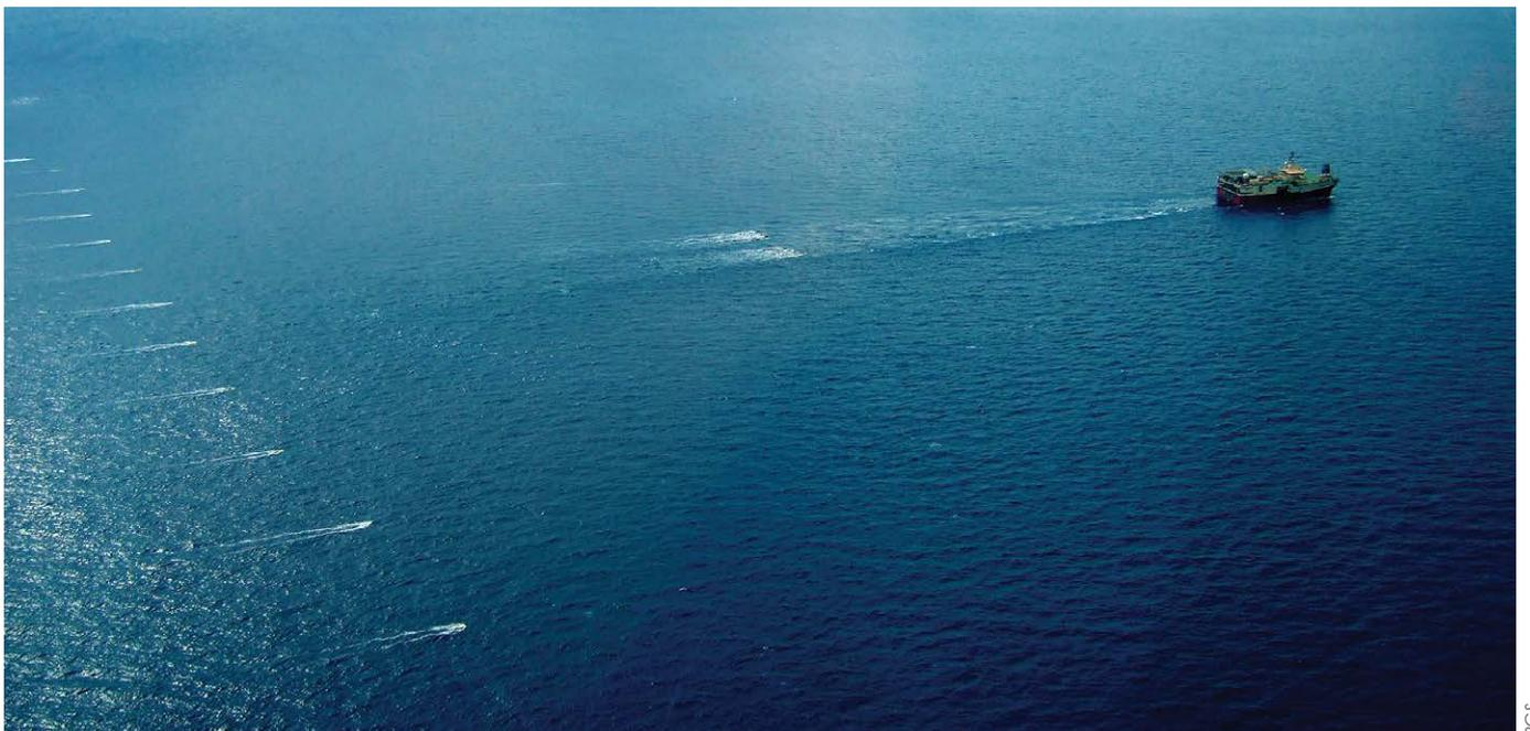
Seismic survey vessels tow airguns as well as the hydrophone-containing ‘streamers’ that may be up to 10 km long.
