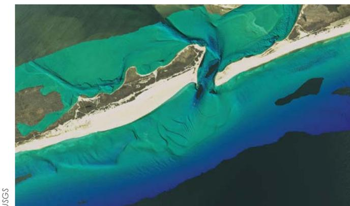
**Airborne lidar bathymetry was used here to identify features in an estuary and nearshore region.**
