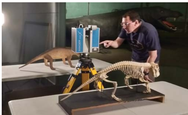
A Zamani Project team member in action, digitising fossil replicas using a 3D laser scanner.
