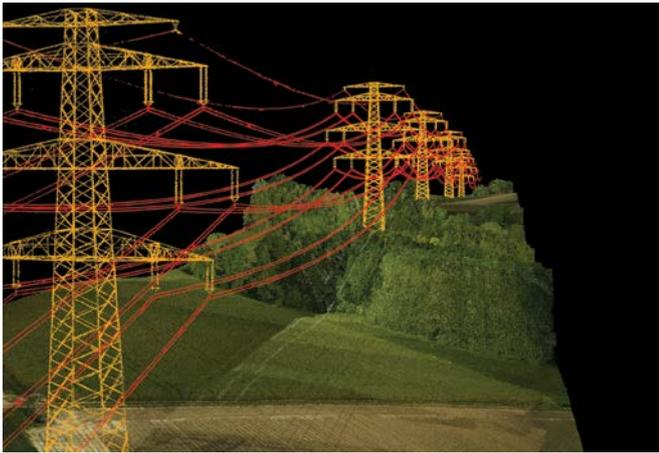
**Inspection of power lines has been taken to a new level with the Siemens SIEAERO service, which relies on drones equipped with highly sensitive lidar sensors, together with smart analytics software that uses artificial intelligence (AI) and machine learning. The service allows for rapid and precise automated detection and assessment of faults and issues along the lines.**
