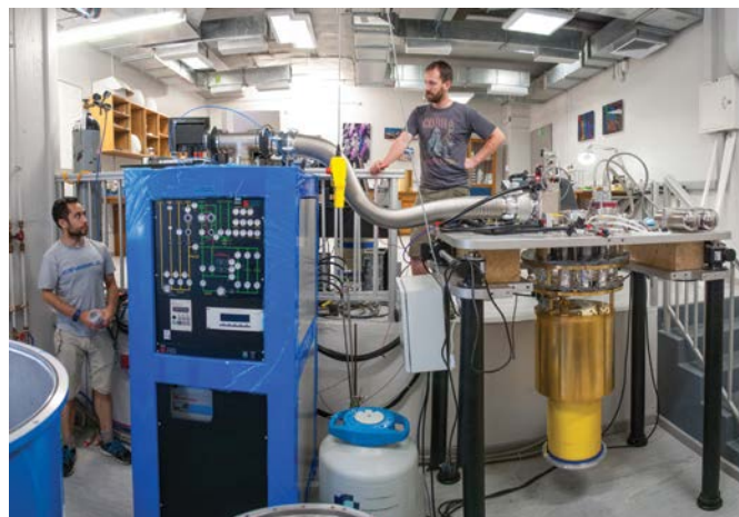
Postdoctoral researchers helped to set up the cryogen-free ^3\text{He} - ^4\text{He} dilution fridge in the UCT Physics Department.
