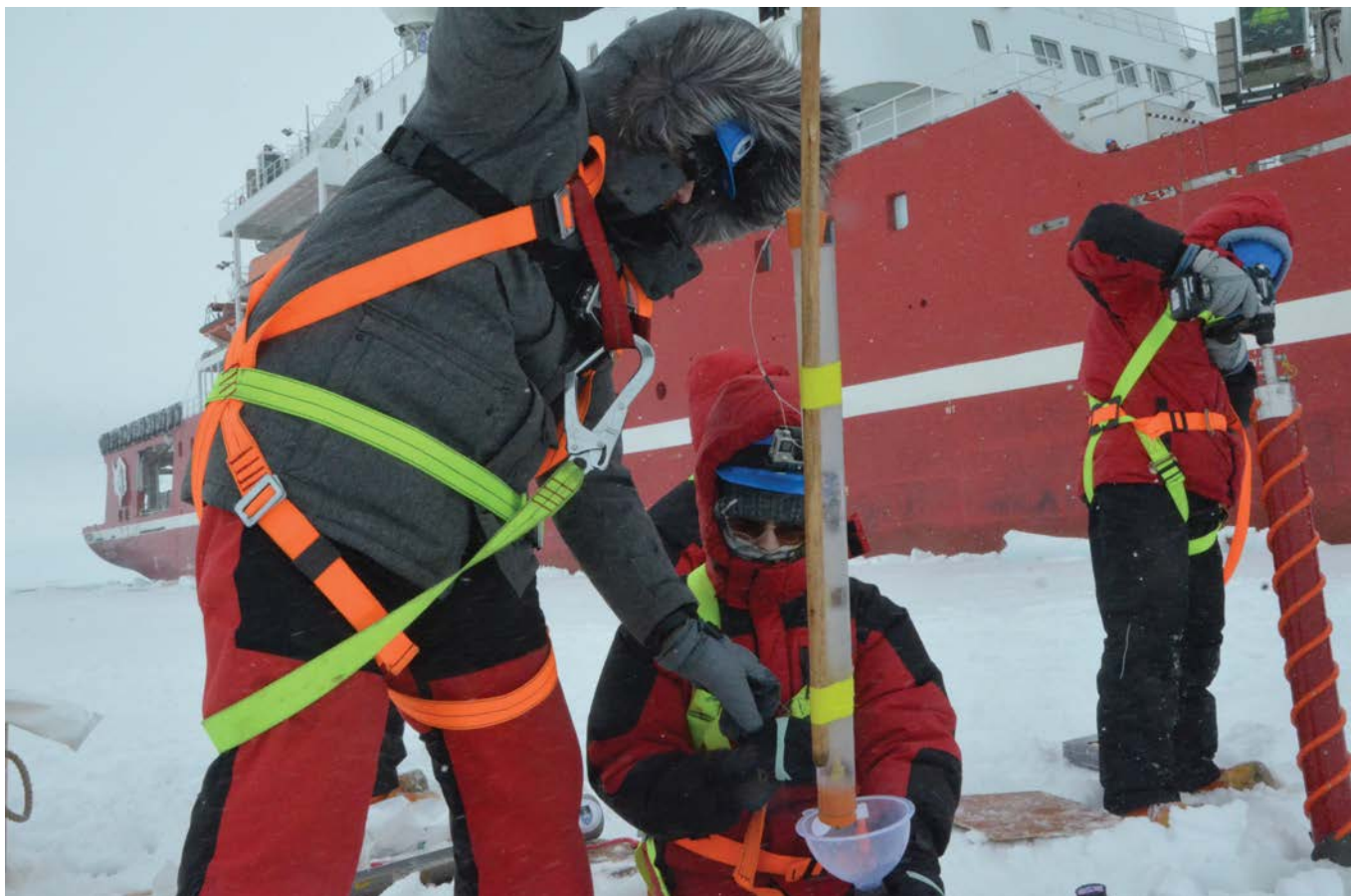
After removal of the cores, water samples are collected from the holes for further analyses, such as nutrient, chlorophyll a and salinity measurements.
