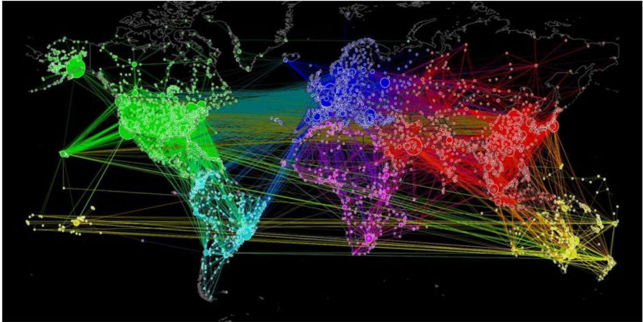
Figure 2: A network visualisation of global air traffic. The hub-and-spoke nature of flight routes point to a small-world structure of the network.
