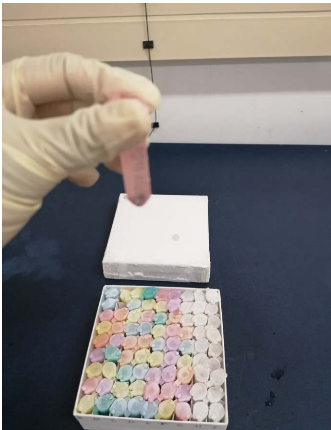
Samples are stored in two-millilitre Eppendorf tubes with a solution of 99.9% ethanol.
