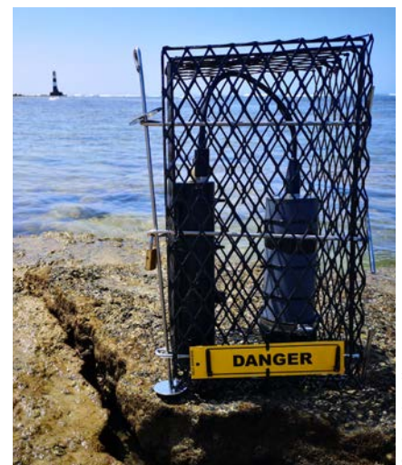
This device, which measures seawater pH and temperature every half hour, is deployed in shallow water in Algoa Bay (Port Elizabeth / Gqeberha) for a few days at a time to monitor ocean acidification.
