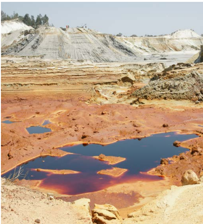
Acid drainage also flows from tailings – the ore residues after mineral processing – and in South Africa this is typically referred to as acid rock drainage (ARD).
