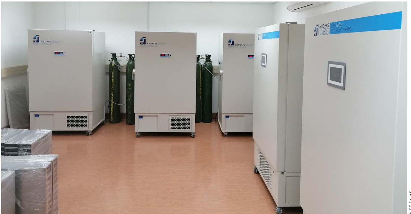
A collection of NRF-SAIAB Biobank minus-80-degree-Celsius upright freezers with back-up CO 2 cylinders.
