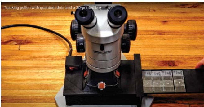
The fluorescent box designed by Corneile for use with a dissection microscope.
