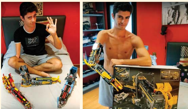
David Aguilar with the first three versions of his prosthetic arm, and with the Lego kit that he used to build ‘Mk-III’.
