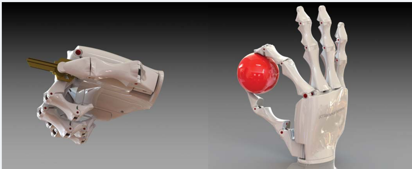
The original Tenim Hand shown here was a mechanically operated prosthesis, controlled by a metal cable linked to a shoulder harness. It is now being updated to an electromechanical prosthesis, activated by electric motors.
