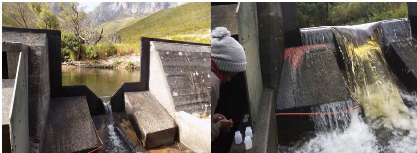
The V-notch gauging weir used to measure streamflow in the Langrivier before and after the rain event.
