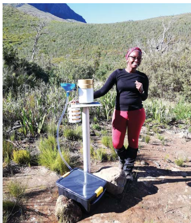
Retang installs the sequential rainfall sampler near the tipping bucket rain gauge.
