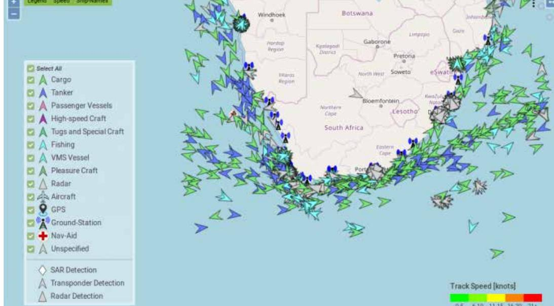
AIS tracking service, which allows fleet managers to keep an eye on their ships as they move around the world's oceans.
