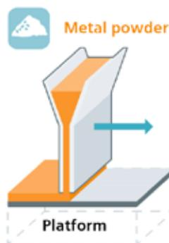
A thin layer of a powder of high performing superalloy is applied.
