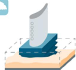
At the end a heat-resistant turbine blade emerges out of the powdered superalloy.
